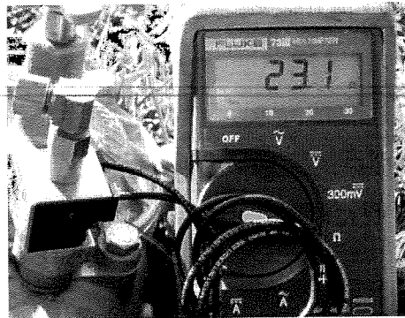
Figure 3. Ohms measurement of a solenoid
