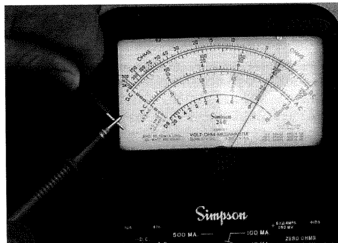
Figure 28. Ground fault test on control wire
