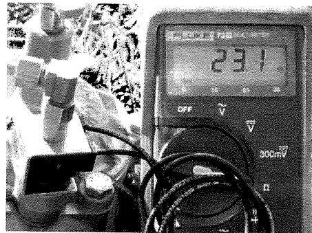
Figure 22. Solenoid resistance reading in ohms
